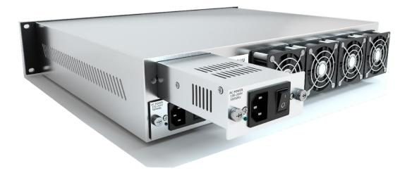
2. Install Power Supply with side Screws. Keep pressing the screws and then
