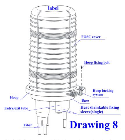
6. Fiber Optic Splice Closures (FOSC) inspecting and testing items
